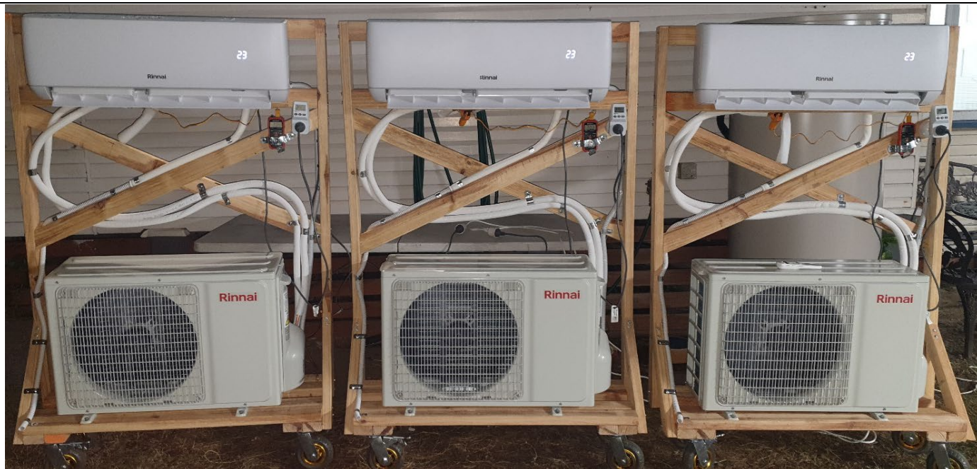
A test rig of three identical split air conditioners for comparing different gas blends against the factory R32 gas.
